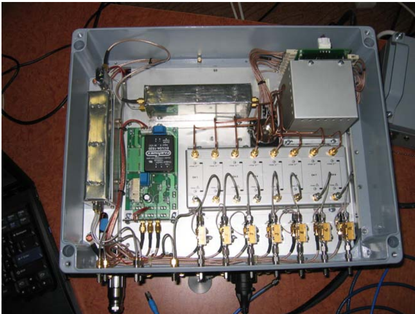
Digital Sampling Converter with open cover. Compartment containing wideband amplifiers
