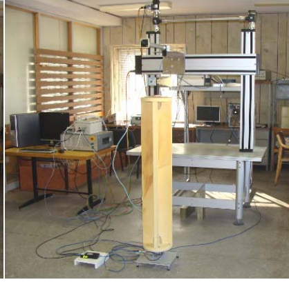
Fig. 3. Cylindrical time-domain antenna measurement setup
