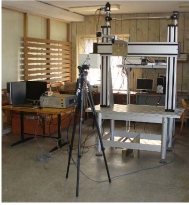
Fig. 2. Planar time-domain near-field antenna measurement setup
